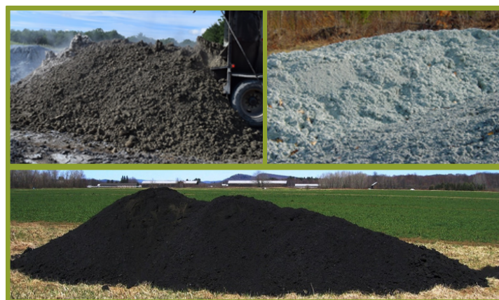
Standard MFT ingredients - Biosolids, Paper Fiber, and Wood Ash.
